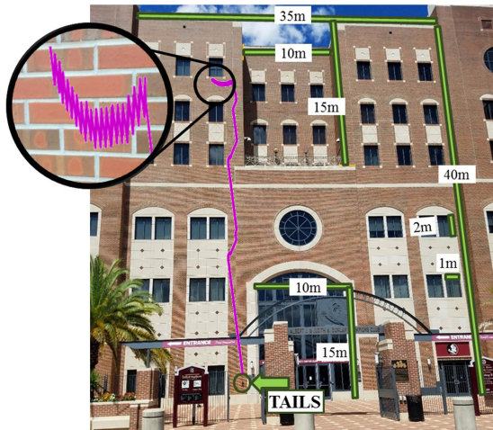
Fig. 7. Theoretically feasible path generated for climbing on a real-world building (FSU's Doak Campbell Stadium).
