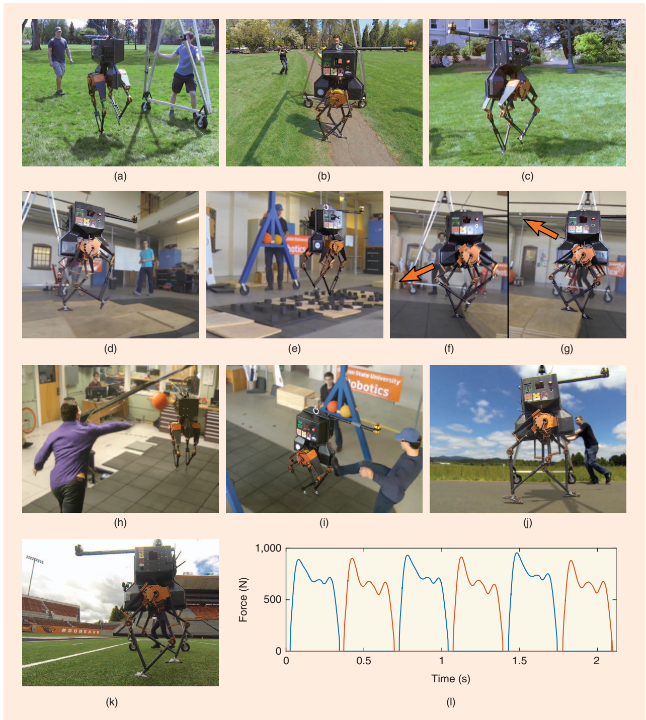
Figure 10. Various experiments with ATRIAS (a) walking on grass, (b) transitioning from pavement to grass, and (c) walking up a 15° grassy slope. In-lab obstacles, (d) transitions between wooden boards and soft foam, (e) randomly structured boards, and (f) stepping up and (g) stepping down a 15-cm platform, all of which were negotiated blindly. External disturbances included (h) repeated dodgeball strikes and (i) strong kicks. High-speed tests included (j) a top speed of 2.5 m/s and (k) a smooth transition from rest to walking to running and back to rest on stadium turf. (l) The plot for the vertical ground-reaction forces for each leg, with gaps between indicating short periods of flight. (Figures courtesy of Christian Hubicki and Patrick Clary.)
