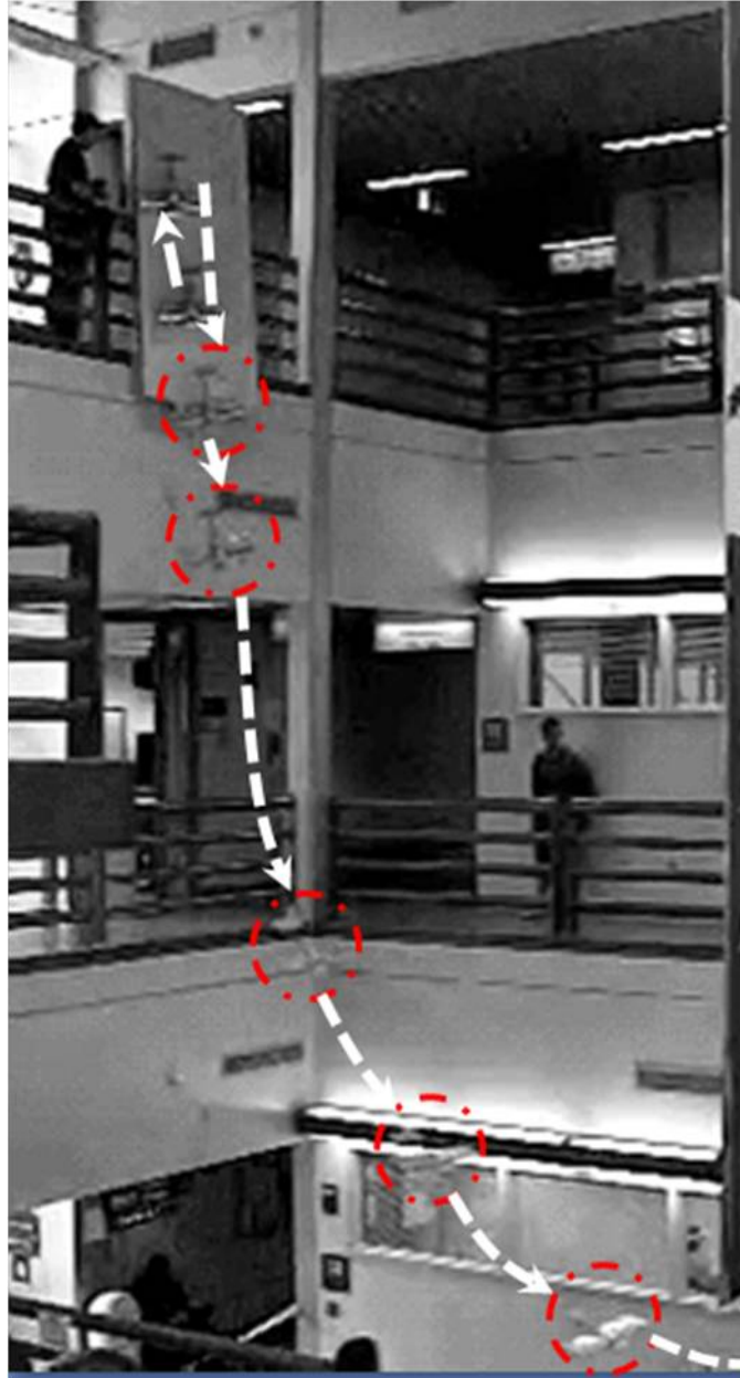
Figure 7.6: Time lapse image of the multi-modal operation of the ICAROS platform. The platform climbs vertically on a prepared climbing surface before detaching and entering a ballistic dive. The platform actuates its rear elevator to transition to a level, horizontal glide path.
