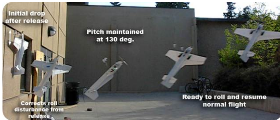
(b) Take off procedure for perching project
