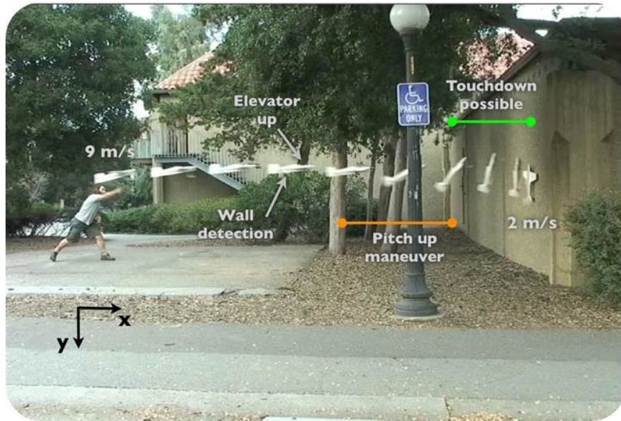
(a) Landing procedure for perching project
