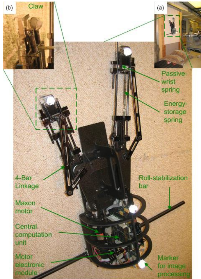
Figure 2.3: The dynamic climbing platform developed by [15] based on the template developed by [28] and discussed in Section 2.1.1.
